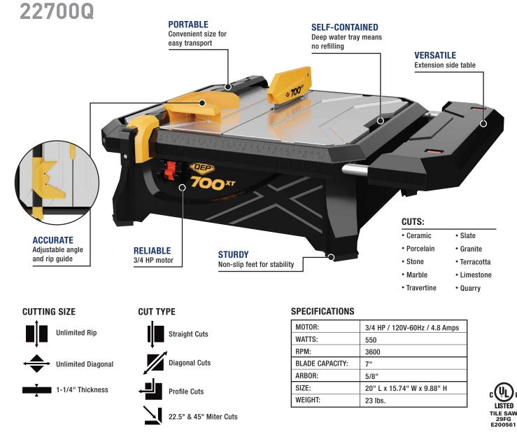
The QEP® 700XT 7" Wet Tile Saw makes straight, diagonal, profile and bevel cuts on a wide array of tile and stone material. The powerful, 3/4 horsepower, 550 Watt motor cuts tile up to 11/4" thick. The included 7" continuous rim diamond blade, table extension, rip guide and angle guide make this wet saw perfect for most cutting jobs. For porcelain and hard tiles, use QEP's Black Widow Blade, 6-7008BW. This cutter includes a wrench to quickly change blades.
