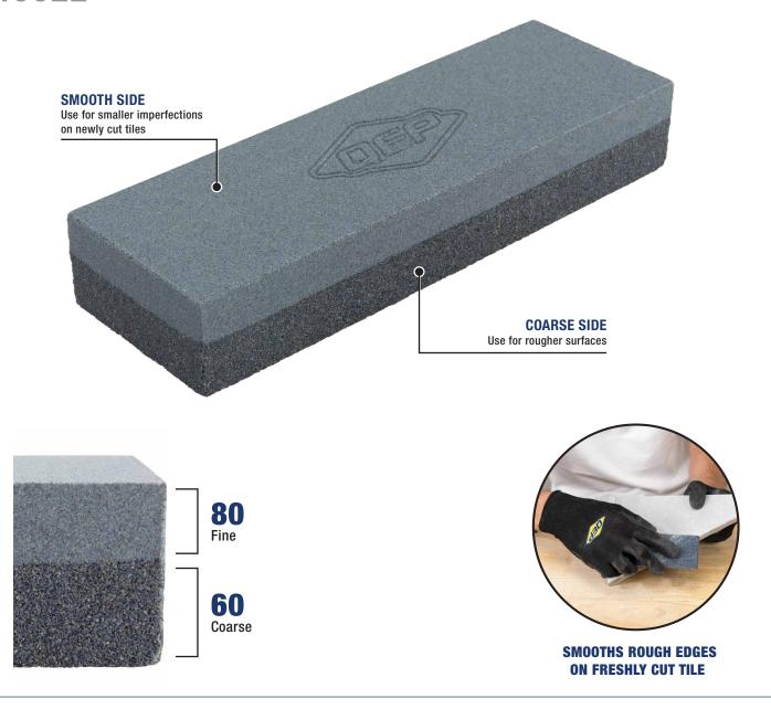
The QEP® Dual Grit Sanding and Rubbing Stone smooths rough edges on freshly cut ceramic and porcelain tile, stone, marble and brick. It features 60 and 80 grit surfaces for medium and fine abrasion. This stone is designed to fit comfortably in your hand for ease of use. It may also be used to remove built up debris on diamond blades.
