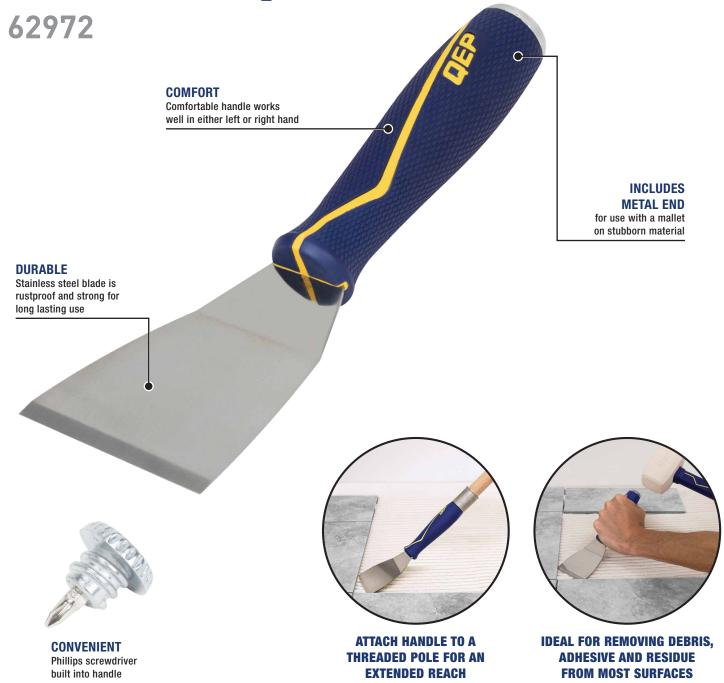
The QEP® 3" Stainless Steel Chisel Scraper is a multifunctional tool that is ideal for removing paint, adhesive and debris from most surfaces. It features a rubber mallet plate for stuborn material. The comfortable rubber handle with non-slip thumb rest makes it easier to use. This durable scraper may also be used to spread materials, including caulk, putty and grout.
