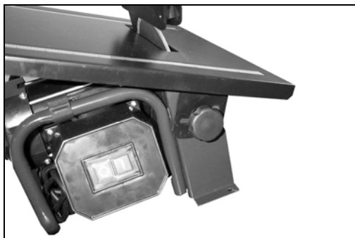
Figure 5: Tilting the table for bevel cutting
